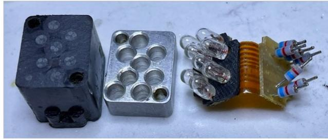
These displays have one lamp per segment and light guides to the front. Some types have built-in diodes and are therefore polarized. So there are some with a common cathode and some with a common anode.
